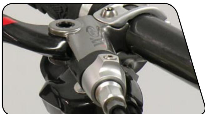
**8** Use the T10 TORX to remove the lever bleed port screw.
