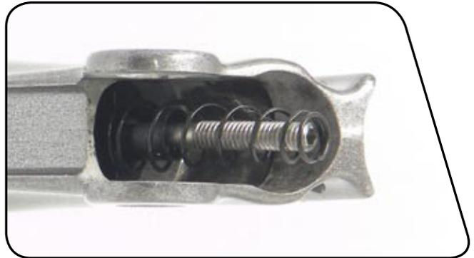
**12** Insert a 2 mm hex wrench through the non-stepped side of the push rod pivot pin and into the reach adjust pushrod. Place the lever blade into the opening of the lever body, then use the 2 mm hex wrench to turn the pushrod counter-clockwise and thread it into the pushrod pivot pin from the stepped side of the pin. Thread the pushrod through the pin until it is flush with the non-stepped side.
