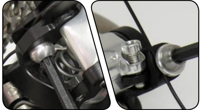
**3** Cut the cable off 6" (15 cm) from the shifter barrel adjuster. Discard the old cable and cable housing.
