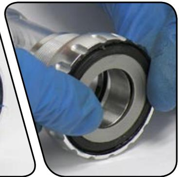
**3** Use calipers to measure your frame's bottom bracket shell width. 68 mm bottom bracket shells require **one** 2.5 mm spacer **on each side** of the bottom bracket shell. 73 mm bottom bracket shells **do not** require spacers.
