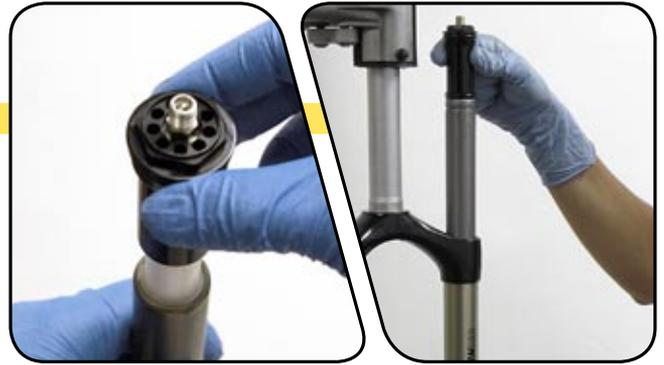
**21** Apply a few drops of medium strength thread lock to the top cap outer threads. Use a 24 mm socket wrench to thread the top cap into the upper tube. Tighten it to 14.6 N·m (130 in-lb).
