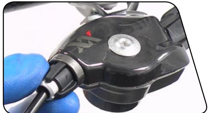
**7** Feed the front shifter cable through the cable housing and cable stops. Run the cable under the cable anchor washer and pull taut.
