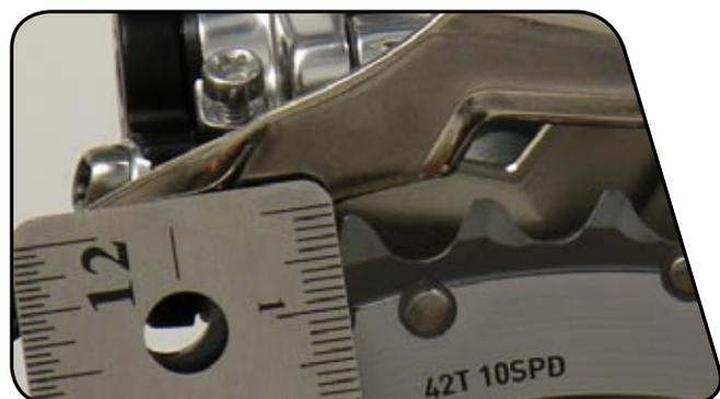
**2** Align the front derailleur cage outer plate to be parallel with the chainrings.
