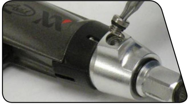
**9** Make sure the fluid in the 1/4 full syringe is pushed all the way to the tip (no air gap!), then thread into the lever bleed port.
