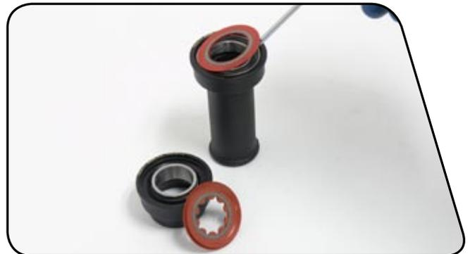
**3** Apply grease to the bottom bracket and frame surfaces as illustrated, including the inside face of the bearing seals, and the wave washer. The seals should be pressed into the bottom bracket cups so that the outer lip seats firmly into the bottom bracket cup groove.
