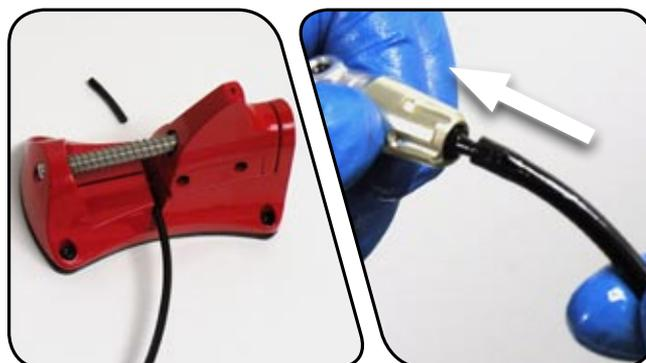
**2 To increase the hydraulic hose length:** Use a sharp knife to carefully cut a slit in the hydraulic hose across the top of the hose barb at the fork crown and the hose barb at the XLoc. Do not scratch the hose barbs.
