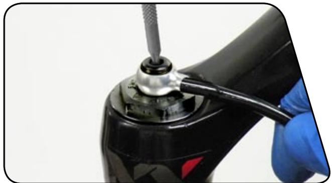
**6** Fill both Speed Lube syringes with 10 ml of 5wt suspension fluid.
