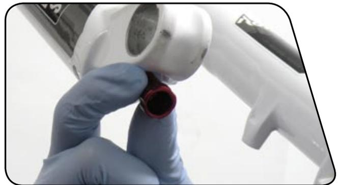
**10** Thread the positive/negative air valve caps onto the air valves.
