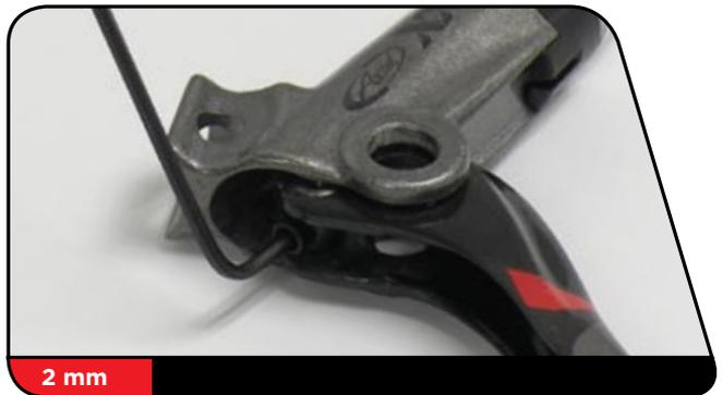
**6** Remove the lever, lever bushings, and piston spring from the lever body.
