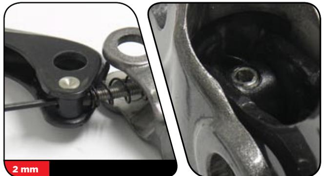
**13** Slide a pivot bushing in between each side of the lever blade and the lever body. Align the holes in the lever body, both bushings, and the lever blade, then slide the press sleeve of the Pivot Pin Press into the holes to maintain alignment.
