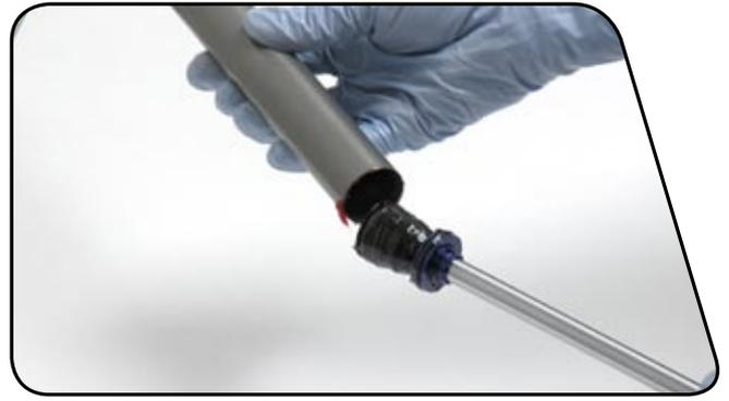
**17** Wipe any remaining grease from the snap ring groove with a clean rag. Use large internal snap ring pliers to secure the snap ring into its groove.
