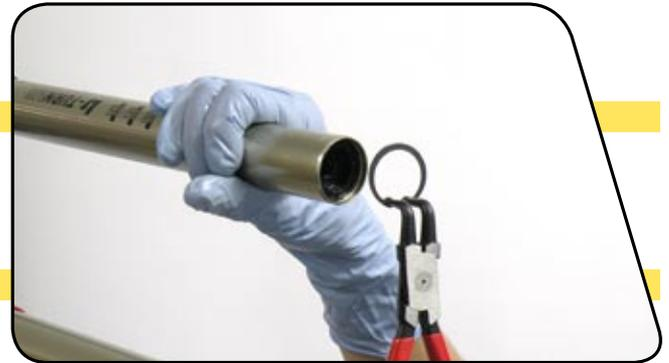
**18** Insert the negative piston retention plate into the end of air tube, stepped side first. Use small external snap ring pliers to re-install the retention plate snap ring.
