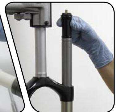
**20** Thread the top cap onto the travel adjustment seal head until the Schrader valve is completely extended from the hole in the center of the top cap.
