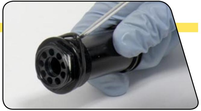
**9** Use small external snap ring pliers to remove the small external snap ring located at the bottom of the air assembly, then remove the negative piston retention plate.
