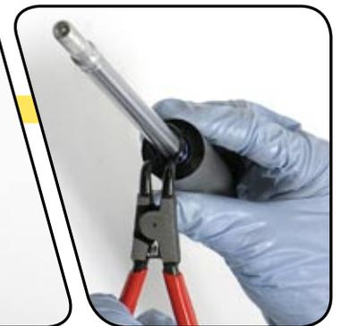
**19** Place the plastic washer over the air valve and seat it against the top of the keys on the travel adjustment shaft. Apply grease to the travel adjustment seal head threads and shaft o-ring.
