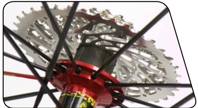
**2** Position the smallest cog on the hub driver. Screw the lockring into the driver.
