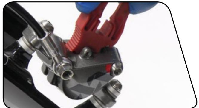
**4** Use the T10 TORX to remove the caliper bleed port screw from the banjo bolt
