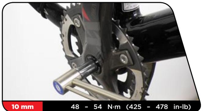
**12** Gently tap the drive side crankarm self extractor bolt with a rubber mallet to fully seat the crankarm.
