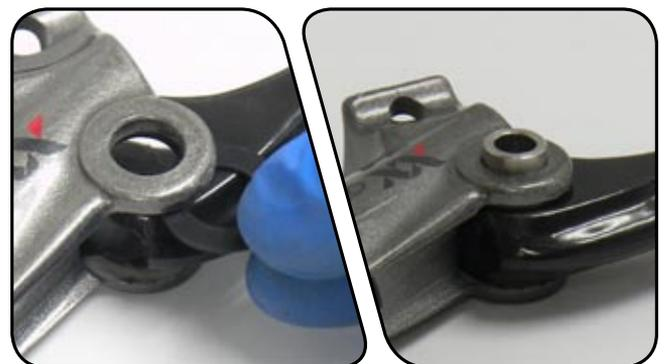
**14** Use the Pivot Pin Press to install the pivot pin into the lever:
