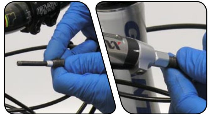
**10** While continuing to push the hose into the hose stop, use an 11 mm open ended wrench to hold the hose stop in place and use an 8 mm open ended wrench to torque the compression nut to 5 N·m (47 in-lb).
