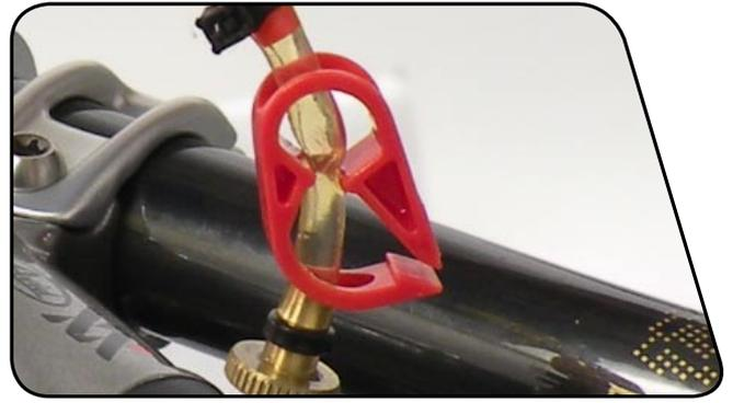
**17** Pull out on the lever syringe plunger to create a vacuum, then gently push in on plunger to pressurize the system. Squeeze and release the brake lever ten times, allowing the lever to snap back to its starting position after squeezing (this helps break loose the bubbles). Repeat this procedure of creating a vacuum at the syringe and squeezing the brake lever ten times until large bubbles stop coming out of the lever.
