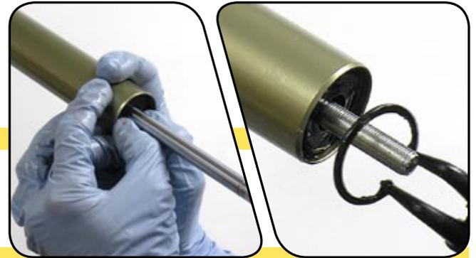
**12** Use isopropyl alcohol and a clean rag to clean the top cap, then apply a small amount of grease to the top cap threads and o-ring. Insert the top cap into the upper tube/crown and hand thread it into the upper tube. Be careful not to damage the top cap o-ring upon installation.
