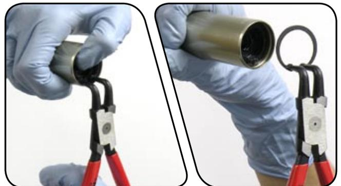
**5** Use a long dowel to remove the base plate from the upper tube. Use a pick to remove the inner and outer base plate o-rings. Apply grease to the new o-rings and install them.
