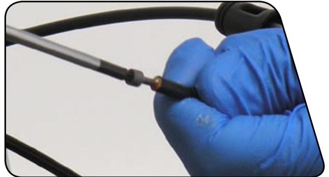
**9** Slide a new compression fitting over the end of the hose with the new hose barb.
