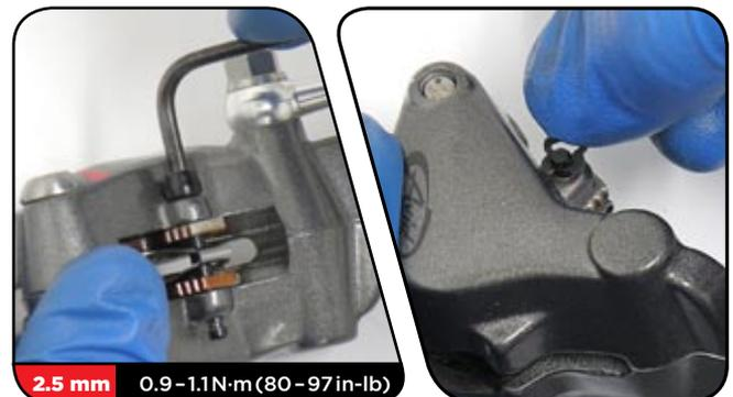
**23** Visually check your work. Inspect the banjo bolt and banjo for any protruding o-rings. If there are any o-rings that are 'squeezed' beyond the outside edges of the banjo or bolt, remove and replace the o-rings, and then repeat the installation process.
