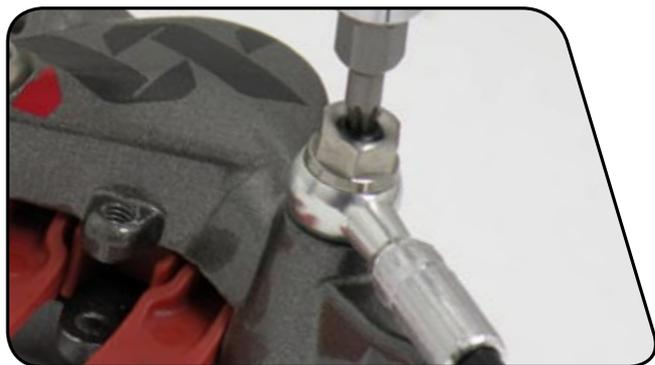
**5** Make sure the fluid in the 1/2 full syringe is pushed all the way to the tip (no air gap!), then thread into the caliper bleed port.
