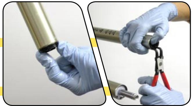
**7** Turn the top cap clockwise to unthread it from the top of the air assembly. Use a pick to remove the plastic washer from inside of the top cap or from the top of the travel adjustment shaft. Set the washer aside.
