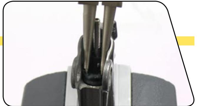
**9** Replace the entire piston/bladder/snap ring assembly with a new assembly. Lubricate the piston/bladder assembly by dipping it into DOT 5.1 fluid.
