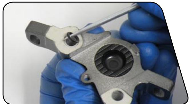
**17** Re-assemble the two caliper body halves. Use a T25 TORX to loosely re-install the caliper body bolt to hold the assembly together.
