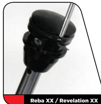
**9** Re-install the negative piston, base plate bumper and base plate onto the Dual Air shaft and thoroughly re-apply grease to the assembly.
