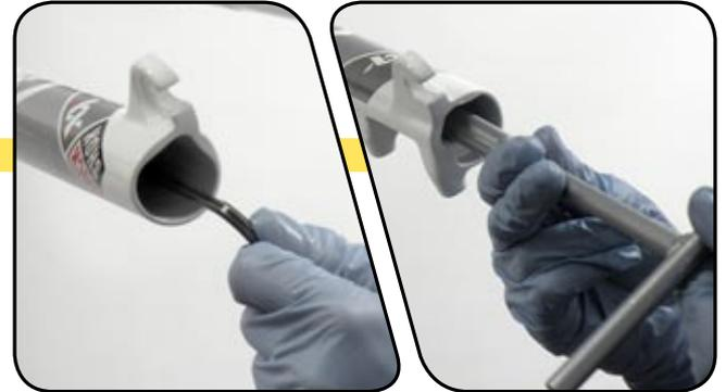
**7** Insert the external rebound damper knob into the rebound damper shaft bolt. Push it in until secure. Adjust as desired.
