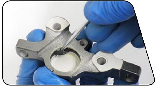
**15** Inspect the caliper pistons for damage and replace if necessary. Re-install the caliper brake pistons into each half of the caliper body. Make sure the piston slots are vertical in the caliper body. (this keeps the fluid slots on the back side of piston lined up with fluid ports).
