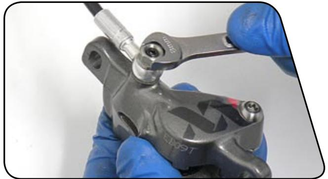
**5** Pull the banjo bolt completely out of caliper. Dump all caliper brake fluid into a container.
