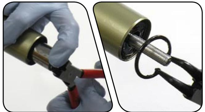
**4** Firmly pull the air shaft down to remove the air spring assembly from the upper tube.
