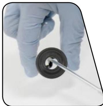
**7** Spray isopropyl alcohol on the rebound damper shaft and wipe it with a clean rag.
