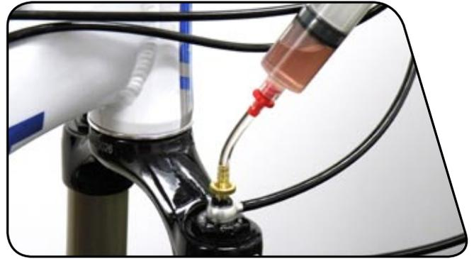
**8** Gently push in the syringe plunger to fill the system with suspension fluid.
