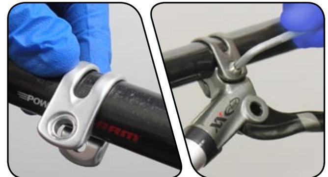
**2** To install the shifter, slide the discreet clamp onto the handlebar, and then install the shifter onto the clamp.
