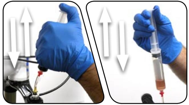
**12** Unthread the syringe from the damper, and use a T10 TORX wrench to re-install the bleed screw into the damper. Use a rag to wipe off any excess suspension fluid.
