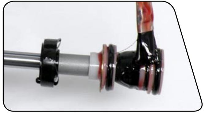
**10** Insert the Dual Air assembly into the upper tube, air piston first, followed by the negative piston and base plate assembly.
