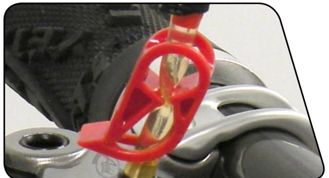
**12** Pull the brake lever all the way to the bar with your finger and hold it there until instructed to release the lever in a later step.
