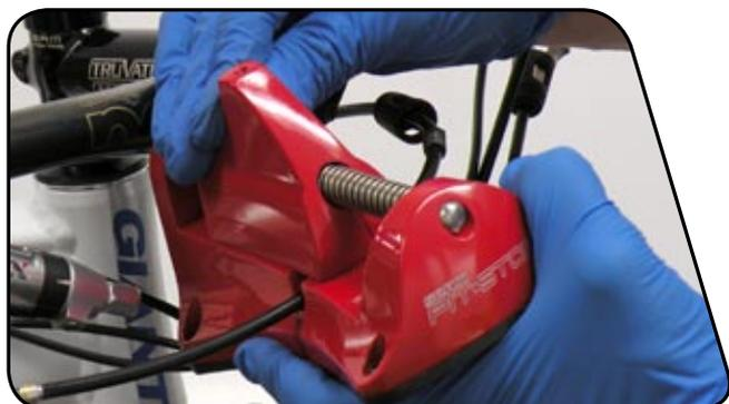
**7** Apply DOT compatible grease to the threads of a new hose barb, the compression fitting outer surfaces and compression nut threads.
