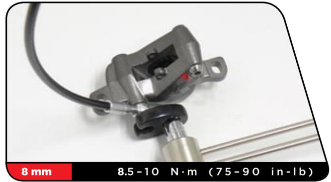
**19** Use a T25 TORX wrench to torque the caliper body bolt to 8.5 - 10 N·m (75-90 in-lb).
