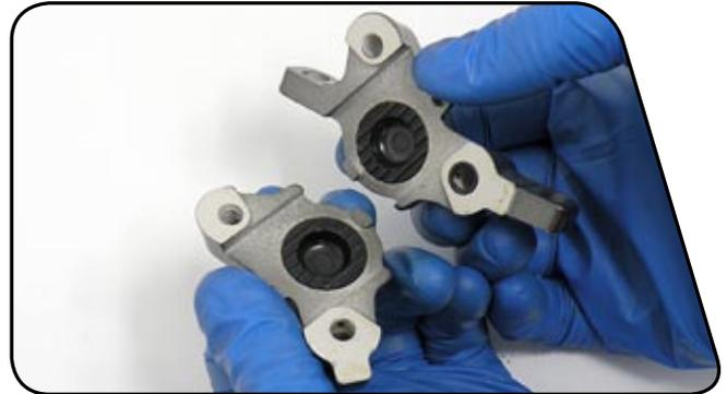
**12** Using a sharp pick, remove the small banjo hole (body half) o-ring.
