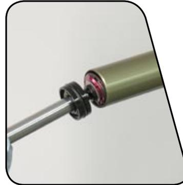
**6** Slide the seal head off the damper shaft and use a pick to remove the inner and outer seal head o-rings. Apply a few drops of Pit-Stop suspension oil to new o-rings and install them.
