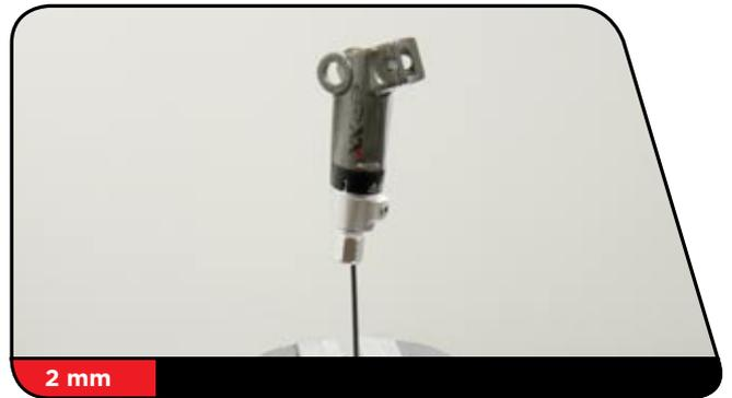
**8** While applying light downward pressure to the lever body, use long snap ring pliers to remove the snap ring in the lever body along with the piston/bladder assembly. Remove the lever body from the hex wrench.
