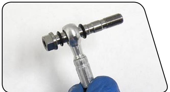
**10** Use a T25 TORX to loosen and remove the caliper body bolt.
