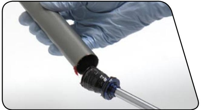
**15** Use a pick to remove the air piston o-ring. Apply grease to the new o-ring and install it.
