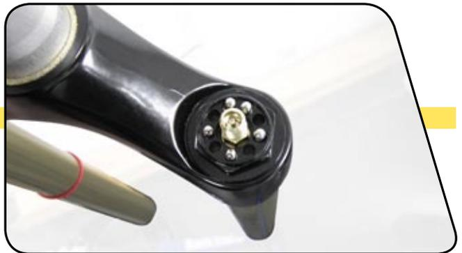
**23** Place the Air U-Turn adjuster knob on the hex-shaped shaft end. Press down on the adjuster knob to access the retaining ring groove below the valve body threads. While pressing down on the knob, use a flat bladed screwdriver to secure the knob retaining ring, from the side, onto the valve body. Make sure retaining ring is inserted into the groove, not the air shaft threads.
