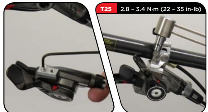
The lower shift lever is infinitely adjustable. Use a T25 TORX wrench to loosen the adjustment bolt. Position the shift lever to suit your ergonomic needs. Hand tighten the adjustment bolt.
