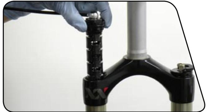
**15** Turn the damper clockwise to thread it into the upper tube. Be careful not to damage the damper top cap o-ring. Continue to thread the top cap down into the upper tube threads and hand tighten. Use a 24 mm flat wrench to tighten to 7.3 N-m (65 in-lb.)
