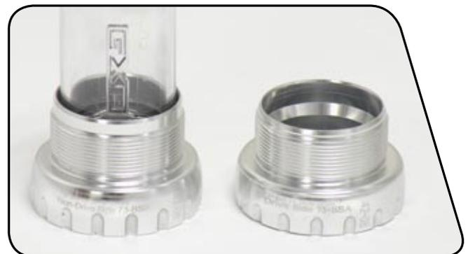
**2** Apply grease to the bottom bracket and frame surfaces as illustrated, including the inside face of the bearing seals. The seals should be pressed into the bottom bracket cups so that the outer lip seats firmly into the bottom bracket cup groove.
