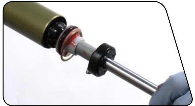
**11** Use your thumb to press the base plate into the upper tube until the snap ring groove is visible. Push the negative air shaft up and into base plate, leaving only the tip of the threaded shaft end protruding from base plate. Use large snap ring pliers to secure the snap ring in its groove. Position the snap ring eyelets on either side of the base plate tab.
