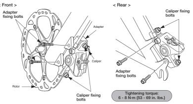
Post mounting type Provisionally install the caliper to the frame (so that the caliper can move sideways), depress the brake lever so that the rotor is being clamped by the pads, and then tighten the caliper fixing bolts
