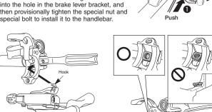
Do not install the nut upside-down. If it is installed upside-down, it will not be possible to secure the brake lever to the handlebars, and damage may occur.
