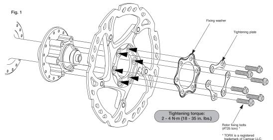
While wearing gloves, apply a force to the rotor to turn it in a clockwise direction as shown in Fig. 2. While doing this, tighten the rotor fixing bolts in the order shown in the illustration.
