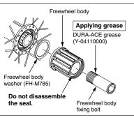
Tightening torque: 45 - 50 N·m {392 - 435 in. lbs.}
