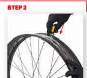
Poke a hole in the tape for the valve.
