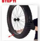
Once the tire is entirely in place, shake the wheel to spread the sealant out within the tire and any leaking areas. Holding the wheel vertical and starting with the valve stem at the bottom, shake wheel to slosh sealent into the bead of the tire. Rotate wheel after each shaking to seal all potential leaks.
