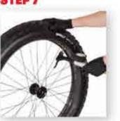
Inflate tube to the tire's recommended pressure. As the tube inflates, the tire will begin to seat and you will hear loud 'bams' as the tire moves into place.
