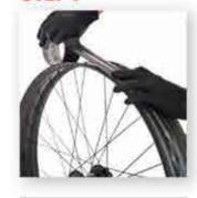
Use one layer of Gorilla Tape " to cover the nipples, leaving about 1 inch of overlap. Press firmly on the tape all the way around the rim to seal the nipples.
