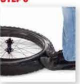
If the tire is too tight, lay the rim on its side, on something soft li.e. grass/carpet/etc.). Without stepping on the carbon, use both of your forefeet to snap the tire into place. Do not pinch the tube.
