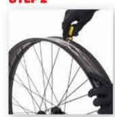
Poke a hole in the tape for the valve.
