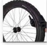
Deflate to your tire manufecturer's recommended pressure. Double check to make sure valve stem is securely tightened to the rim.
