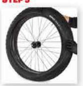
shape, then place it inside the tire. Secure the valve stem in the rim with the locknut. Work the second bead onto the rim, slowly letting air out of the tube as you go around to allow room for the bead. You should be able to do this without tools.
