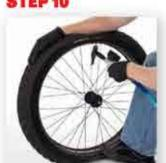
If air is still escaping and the tire beads do not seet on the rim, knock the beads back entirely into the rim channels and add another Inflatoband to each side. Removing the valve core increases air flow to the tire and can help with mounting.
