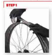
Use one layer of Gorilla Tape™ to cover the nipples, leaving about 1 inch of overlap, Press firmly on the tape all the way around the rim to seal the nipples.
