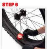
Snap 80% of the second bead into its channel. Leave enough lip to add tire sealant. Add four scoops (recommended, -240 mL total) of tire sealant into the tire.
