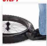
Finish snapping the rest of the second bead into the channel. You should be able to do this without tools. If the tire is too tight, lay the rim on its side, on something soft (i.e. grass/carpet/etc.). Without stepping on the carbon, use both of your forefeet to snap the tire into place.
