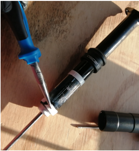
6. Delicately remove the upper and lower bushing and collar. Note the orientation of the lower bushing. This is important for reassembly.
