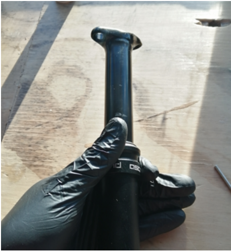
5. Unscrew the collar and remove the stanchion from the post.
