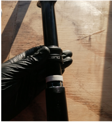
5. Unscrew the collar and remove the stanchion from the post.
