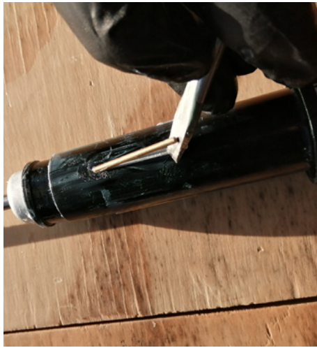
7. Using a pick or a sharp flat headed screwdriver gently lift the brass pins.
