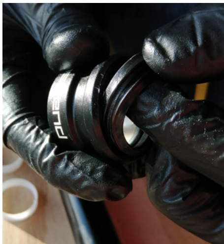
9. Disassemble the collar - remove the metal retaining ring and then lift out the rubber seal.
