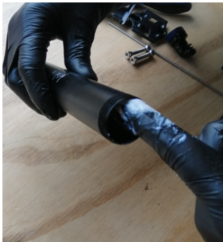
10. Lubricate the inner of the seat post tube.
