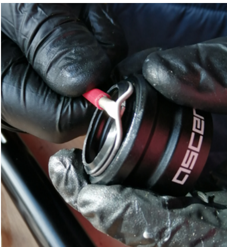
9. Disassemble the collar - remove the metal retaining ring and then lift out the rubber seal.
